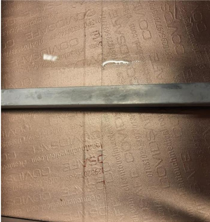
Figure 7. Test 2, additional weights on the basic membrane brushes. Test time 200 brushes. Surface broken at the tape seam.
