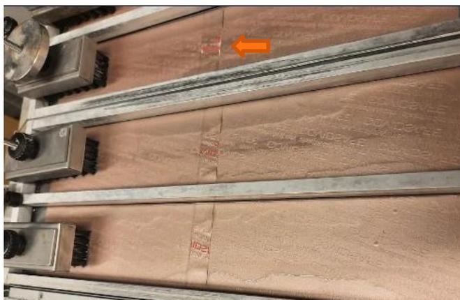
Figure 13. 133 brushes. In the basic brushing, text appears on the embossed part. With additional weights (top groove), the coating has punctured on the embossed part and the base has become visible.
