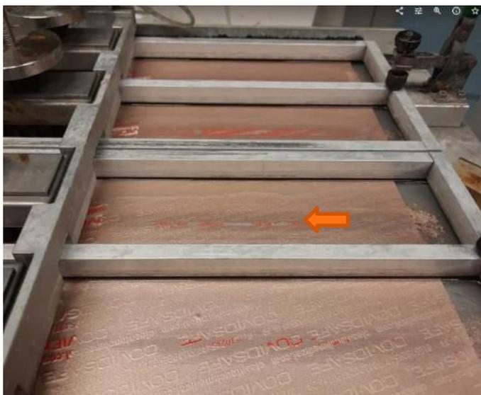
Figure 16. 399 brushes. Coating is slightly punctured and white base appears in basic brushing. Loose coating precipitation begin to accumulate at the ends of the brushing path.
