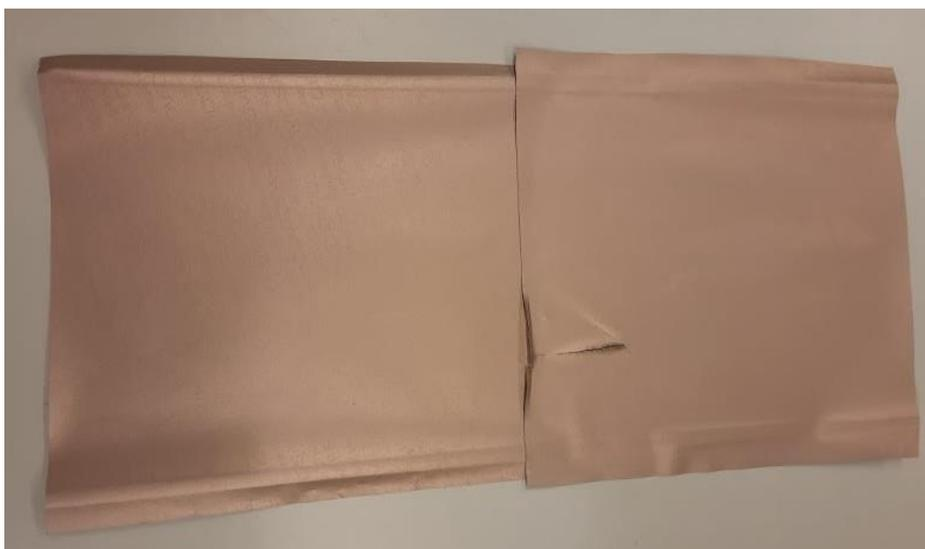
Figure 11. Test 2. Membrane with additive 4000 brushes. No visible changes on the membrane surface.
