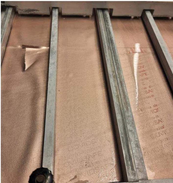
Figure 10. Test 2. Membrane with additive 3000 brushes. The membrane is torn at the tape seam. No visible changes on the membrane surface.
