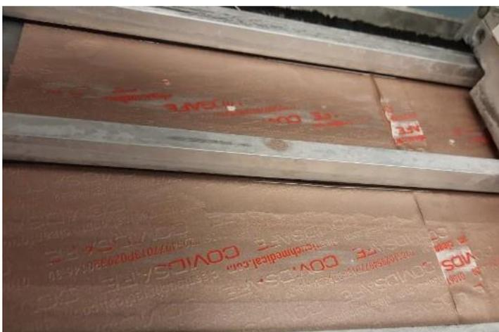
Figure 15. 360 brushes. Coating brushed with additional weights has punctured and white base is visible.
