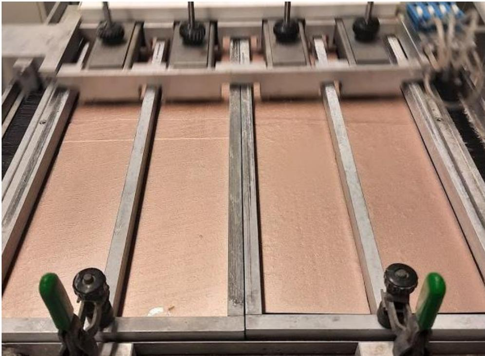
Figure 2. Test 1. Membrane with additive on the left and basic membrane on the right. Test time 200 brushes. There are no visible changes in either membrane.
